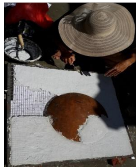
Figure 2.4 Clay Bonding Process on Skillet Construction with Combination of Filter Wire and Iron Plate (Bendi Yudha Dok. 2017)
