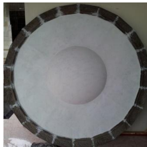
Figure 3.5 Results of Clay Attachment to Pan Construction with a Combination of Filter Wire and Iron Plate, Then Sun-dried (Bendi Yudha Dok. 2017)
