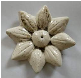
(Source: Diatmika, 2017) Figure 16. White glaze with 20% sand
