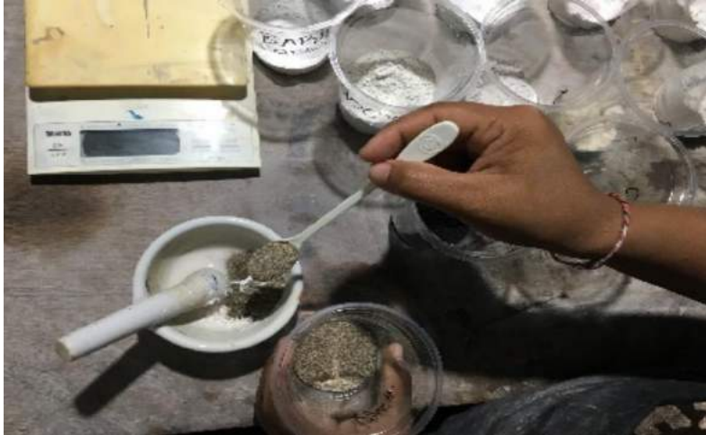
Figure 5. The process of mixing glaze materials
