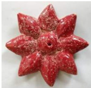
Figure 10. Red glaze with 20% sand
