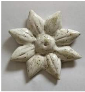
(Source: Diatmika, 2017) Figure 15. White glaze with 10% sand
