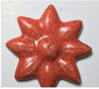
Figure 9. Red glaze with 10% sand
