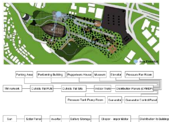
[Source: Herlambang, 2023] Figure 22. Electrical Concept
